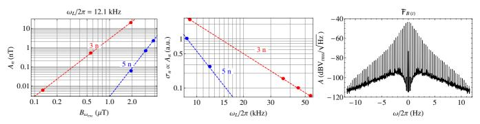
**Figure 1:** Left and central graphs show the  $A_n \propto B_{\omega_{exc}}^n$  and  $\sigma_n \propto \omega_L^{-(n-1)}$  dependencies of the multiphoton process, respectively. The right graph shows the Fourier spectrum of a 157 Hz square-wave modulated B(t) field measured by a self-oscillating magnetometer.
