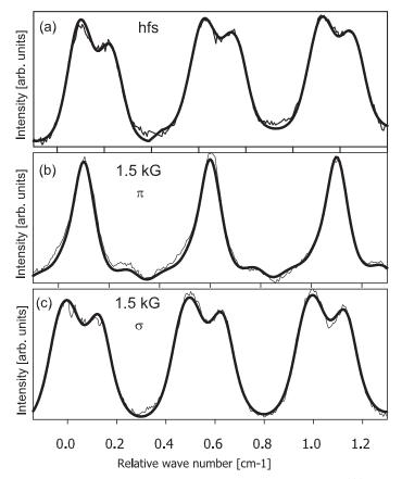
**Figure 1:** The recorded hyperfine structure of the 792.5 nm line of  ${}^{123}Sb$  I (a) and Zeeman patterns  $\pi$ -view (b) and  $\sigma$ -view (c) at 1.50 kG magnetic field. The thin line represents the experimental trace and the thick line shows the computer-generated contour.
