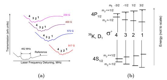
**Figure 1:** (a) Transmission spectrum of <sup>39</sup>K vapor contained in the nano-cell with L = 770 nm for B = 230, 400, 572 and 917 G and  $\sigma^+$  excitation. (b) The diagram of the hyperfine structure of the  $D_1$  line of the <sup>39</sup>K HPB regime, the selection rules are  $\Delta m_J = 1, \Delta m_I = 0$ .
